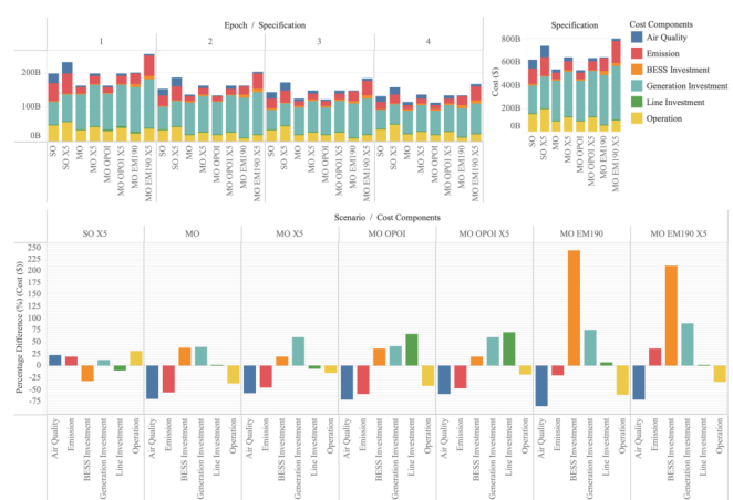
Fig. 26: Optimal costs with varying specifications, with operational scenarios from [47]. Top : Costs across epochs and model specifications. Bottom left : Cost comparisons across model specifications considering SO as the baseline. Bottom right : Total costs across model specifications. X5 denotes consideration of extreme scenarios.
