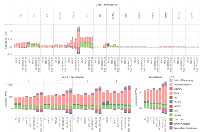
Fig. 13: Optimal generation decisions with varying specifications, with operational scenarios from [47]. Top : Across existing onshore zones and model specifications. Bottom left : Across epochs and model specifications. Bottom right : Total across model specifications. X5 denotes consideration of extreme scenarios.
